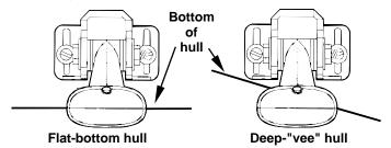
Align transducer centerline with hull bottom and attach to transom.
